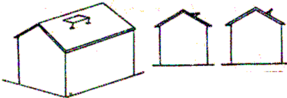
RAISED PANEL MOUNTED PARALLEL TO PEAK
